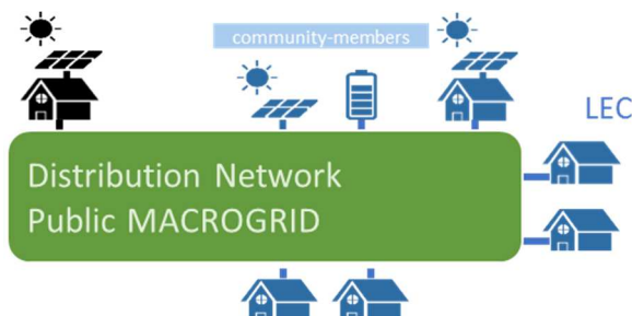
Figure 3 Implementation solution 2 for EC-network
