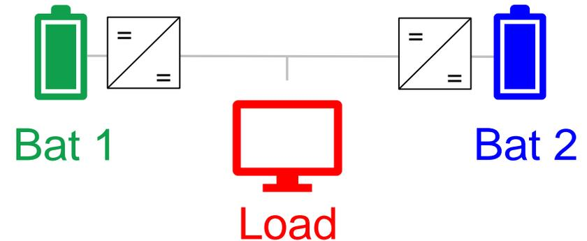
→ Load supply and state-of-charge balancing between the 2 batteries
