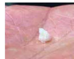
Figure 1. Environmentally friendly hydrogen clathrate hydrate on a palm warming up and melting.
