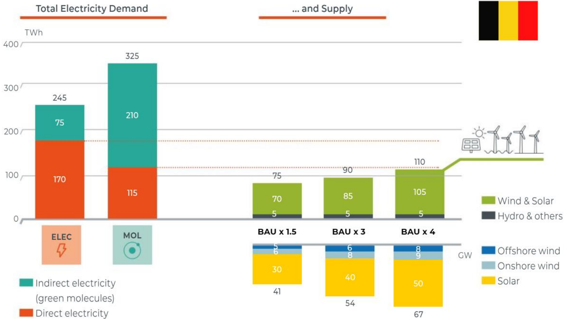
FIGURE 10: COMPARISON BETWEEN THE TOTAL ELECTRICITY DEMAND AND THE ELECTRICITY SUPPLY FOR BOTH TRANSFORMATION PATHWAYS AND ALL THREE SUPPLY SCENARIOS FOR BELGIUM IN 2050
