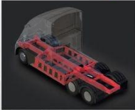
Purpose designed electric truck chassis
